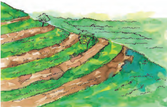
Continuous contour trenches (CCT)
