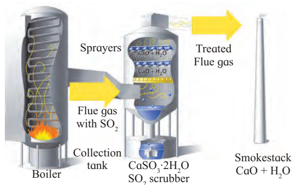
Fig. 15.5 : Exhaust gas Scrubber
