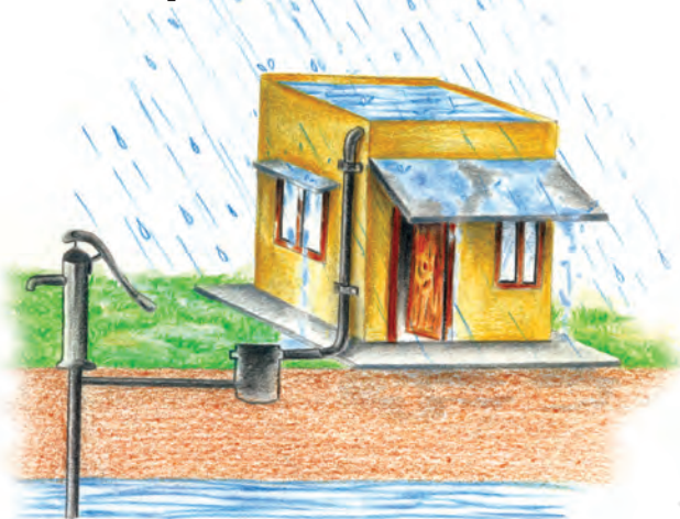
(a) Recharge through Hand Pump
